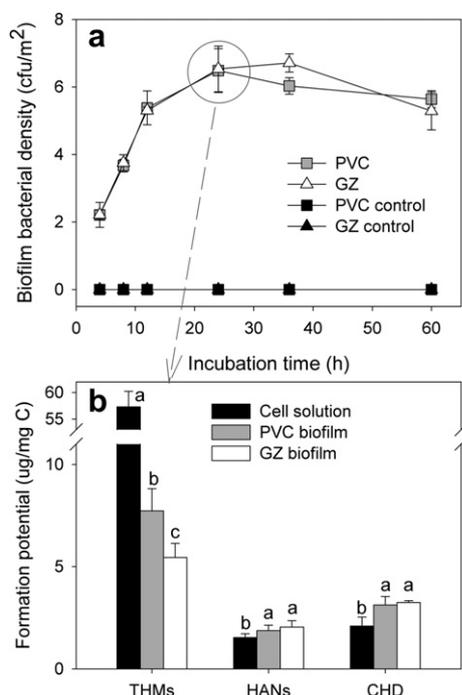
**Fig. 3 – Biofilms formation of *Pseudomonas aeruginosa* on polyvinyl chloride (PVC) and galvanized zinc (GZ) surfaces changed with incubation time (a) and the disinfection byproduct formation potentials of 24-h biofilms compared to that of the pure *P. aeruginosa* cell solution (b). All error bars indicated the standard deviation of 3 replicates.**
