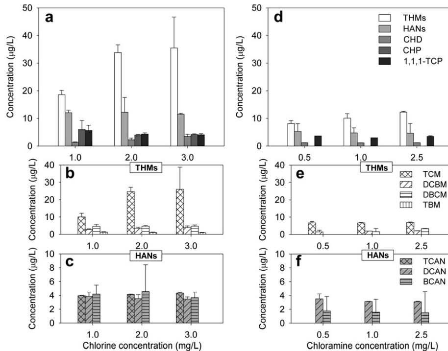
**Fig. 1 – Disinfection byproduct formation after 1 h chlorination and chloramination of pure *Escherichia coli* solution. THMs, HANs and CHD refer to trihalomethanes, halo-acetonitriles and chloral hydrate, respectively. All error bars indicated the standard deviation of 12 replicates.**
