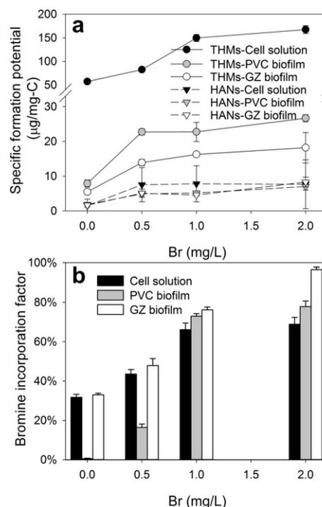
**Fig. 4 – Trihalomethane and haloacetonitrile formation potentials of the *P. aeruginosa* biofilms in the presence of bromide (a), and the bromine incorporation fraction of trihalomethanes changed with increasing bromide concentration (b). All error bars indicated the standard deviation of 3 replicates.**
