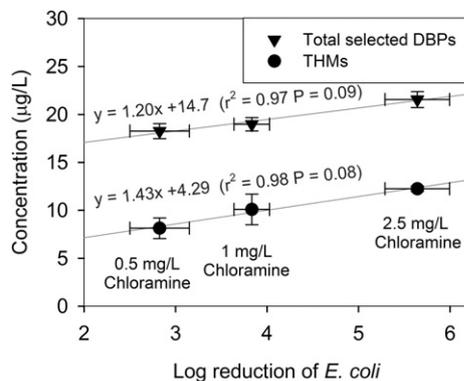
**Fig. 2 – Correlations of total DBPs and trihalomethanes (THMs) formation with the log reduction of *E. coli* after 1 h chloramination. All error bars indicated the standard deviation of 12 replicates.**
